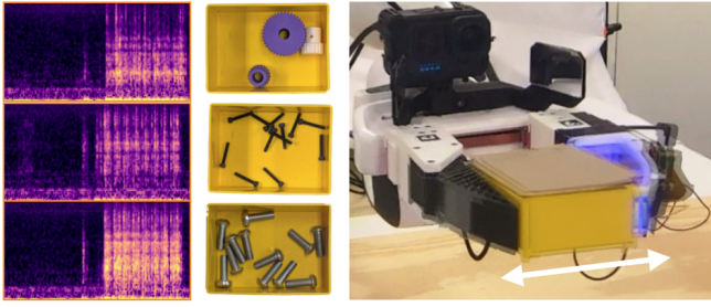
Fig. 6: Audio signals (left) generated by shaking gears, thin screws, and thick screws (middle) with the robot arm (right) enable classification of visually occluded objects, substantially outperforming vision and touch.
